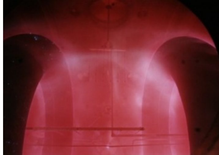
A plasma discharge in MRX. The two flux cores and magnetic diagnostics are visible.
