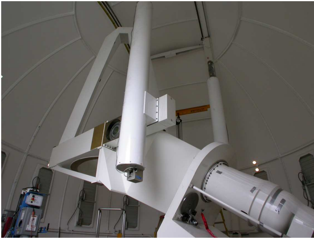
Figure 2: The NST equatorial mount, mirror cell, counterweights (for right ascension balance), and tower to secondary.???UPDATE???
