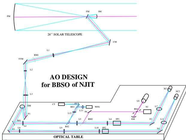
**Fig. 1.** Optical design for the AO system of BBSO's 65 cm vacuum telescope.
