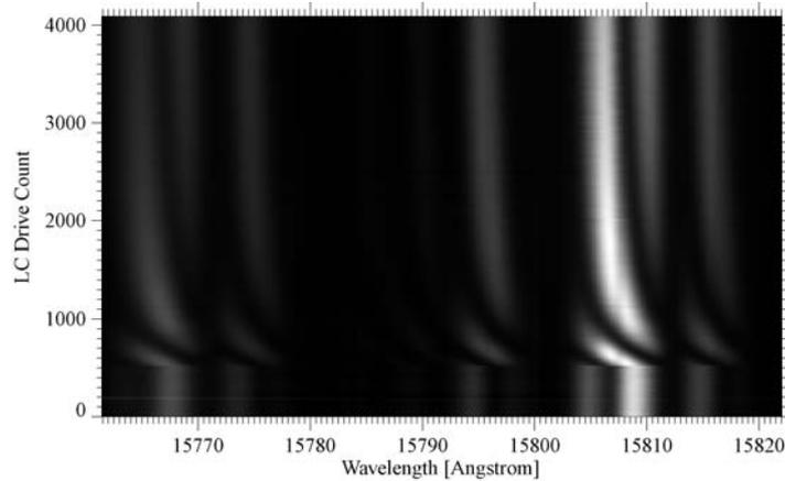
*Figure 3.* The transmission of the thickest module  $M_1$  as a function of drive voltage  $V$  and wavelength  $\lambda$ . The retardance of LCVR does not have any response in the range of 0–500 counts. The *horizontal slices* along the  $x$ -axis present the transmission profiles under different drive voltage. The *vertical slices* along the  $y$ -axis present the calibration curves as transmission vs. drive voltage under  $32.0^{\circ}\text{C}$ .
