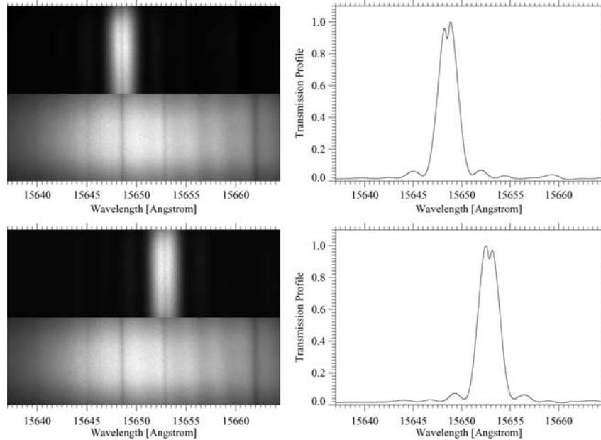
*Figure 4.* The calibration results and transmission profiles when tuned to Fe I 15648.5 Å and Fe I 15652.9 Å spectral lines. (*Left panel*) The transmission bandpass of the spectrograph including or excluding the filter system in the calibration optical path. (*Right panel*) The corresponding transmission profiles. The concave centering at the peak shows the core of the spectral line.
